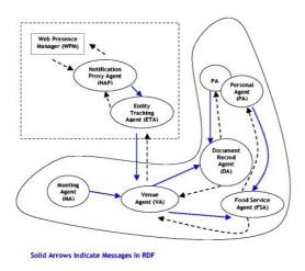
Fig. 1. An overview of the CoolAgent RS architecture
