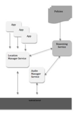
Fig. 2. In this sketch of our prototype architecture, arrows denotes the steps involved and the information flow among the components.
