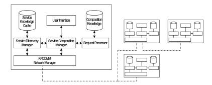
Figure 2. System Components in Anamika Reactive Service Composition Architecture
